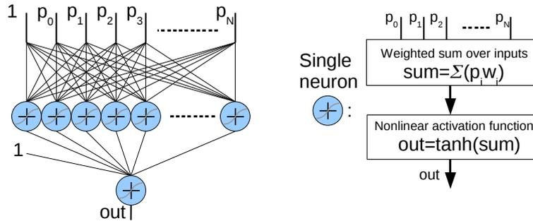
Figure 1: Schema of predictor blending with a 1-layer neural network. The net takes a constant bias and the  $N$  predictions as input. The output is given by the evaluation of the neural network with the trained weights.
